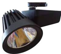
LED-spotlight with passive cooling system. Die cast aluminium body, powder coat painted. Integral electronic driver. Integral heatsink. Rotation 365°. Vertical adjustment +/- 90°. Track mounted with 3-circuit adapter. Voltage 230V.
